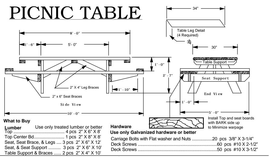
First built two A-shaped end braces to provide legs for supports for both top and seats. Legs are 2" X 6" X 34" long, with a 3-1/4" diagonal cut at each end to accommodate slant for legs (cut from a 12' board). The seat supports are two 2" X 6" 's 60" long (cut from a 12' board). Use two 2" X 4"'s 30' long for table support.
